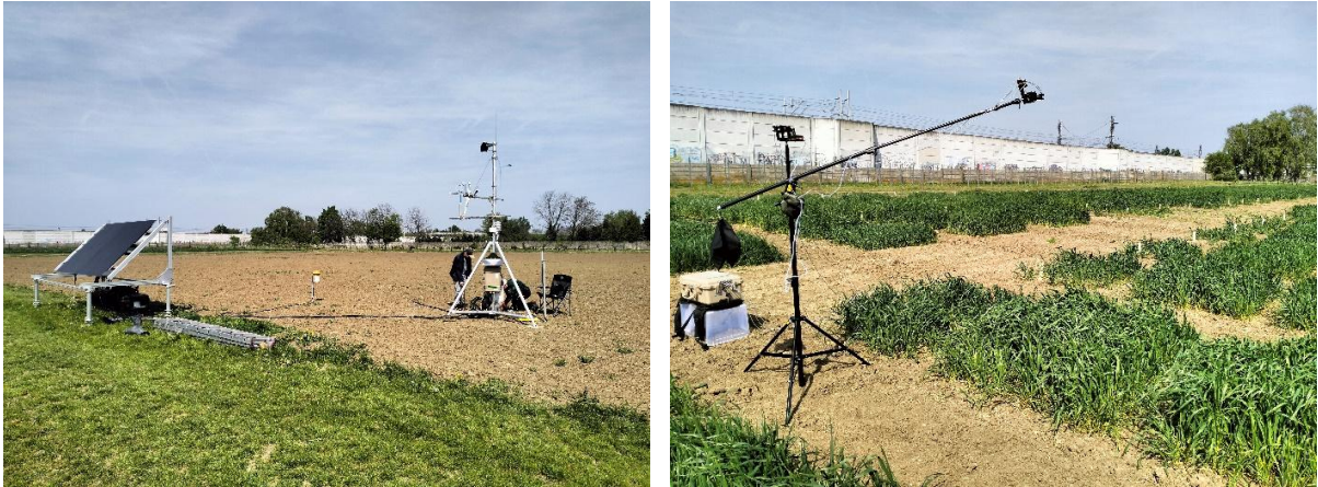
Figure 5.7. Field Cal/Val infrastructure supporting ESA FLEX mission at VÚRV Piešťany. Left: Flux tower (LI-Cor Env.) with FLOX box (JB Hyperspectral) continuous measurements. Right: Mobile FLOX box for ambient SIF measurements.
