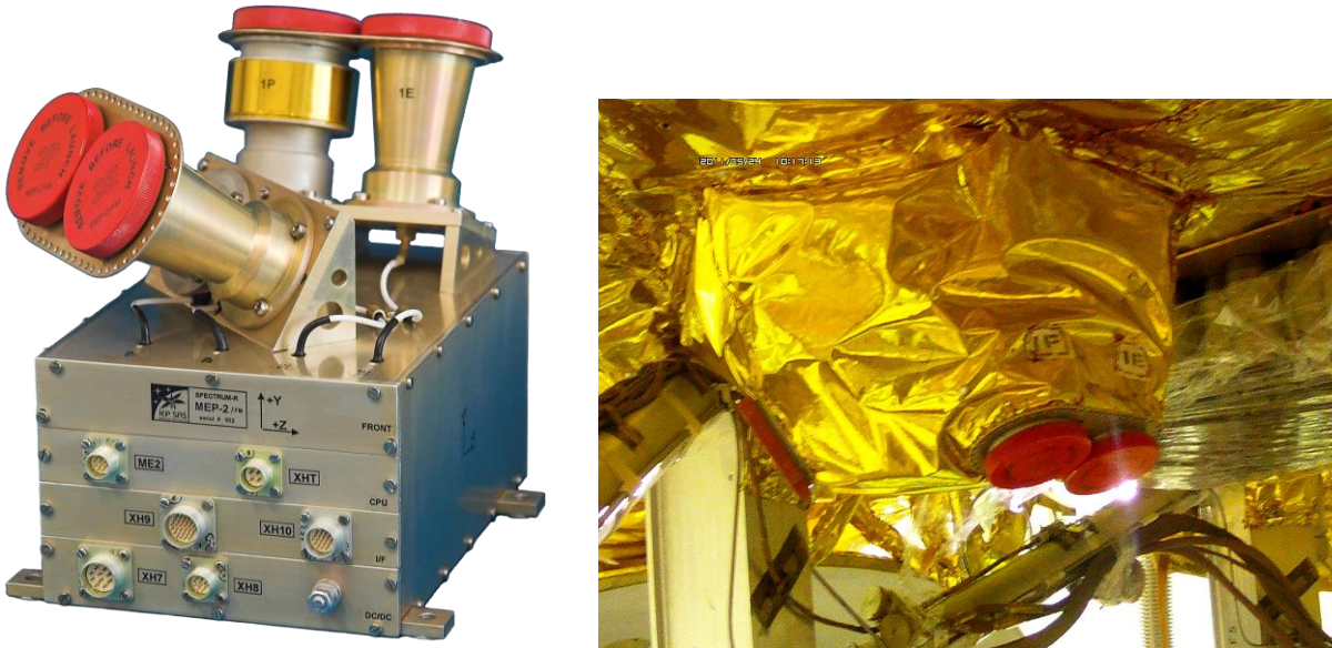
Figure 1.1. Energetic particle spectrometer MEP-2. The configuration on delivery and after installation on board of the space observatory Spektr-R (Radioastron).
