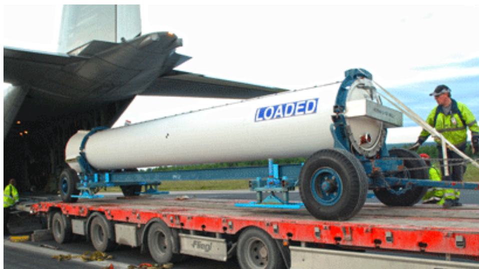
Figure 3.3. Nine meter long Castor IVB rocket motor for MAXUS 9 filled with 10 tonnes of solid propellant.
