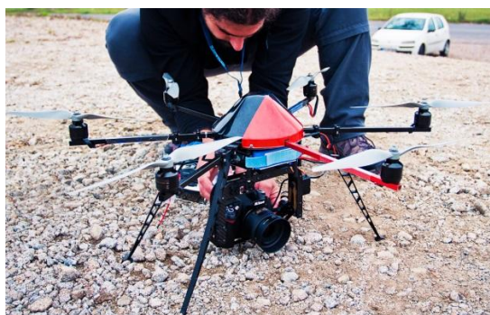
Figure 4.3 An example of multirotor UAV. Six-rotor remotely controlled flying platform with Nikon D90 DSLR + Nikon 35mm F1,8G AF-S DX lens.
