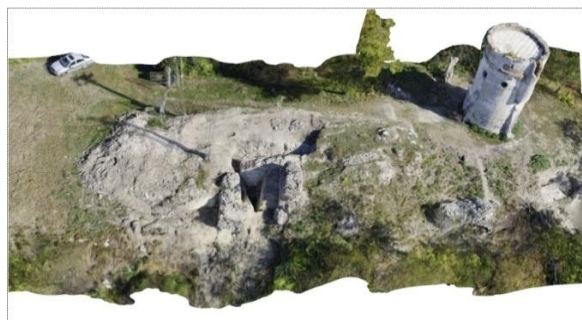
Figure 4.6 Photorealistic model of archaeological site of Čeklís. Model was created from aerial images and ground images in Agisoft PhotoScan.
