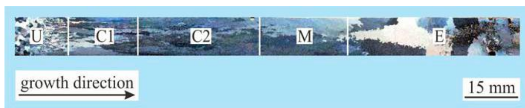
Figure 3.9. Typical macrostructure of longitudinal section of sample prepared by power down technique in Bridgman type apparatus.
