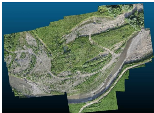
Figure 4.4 A part of ortophoto mosaic of avulsion channel of Ondava river near Stropkov, processed in Airphoto SE. Captured area is about 3.5 ha. Total number of orthorectified pictures – 67 taken from altitude of 70 m. Pixel resolution is 2cm and positional precision of area is subdecimetre.
