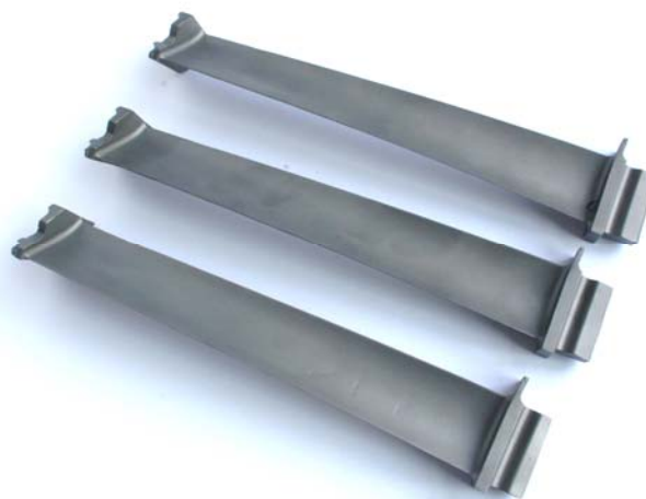
Fig. 1. Centrifugally cast low pressure turbine blades from TiAl based alloy by the coordinator of the project GRADECET - ACCESS, Germany.
