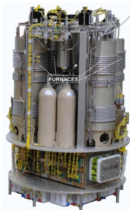
Fig. 5. Designed furnace module for sounding rocket mission MAXUS-9.
