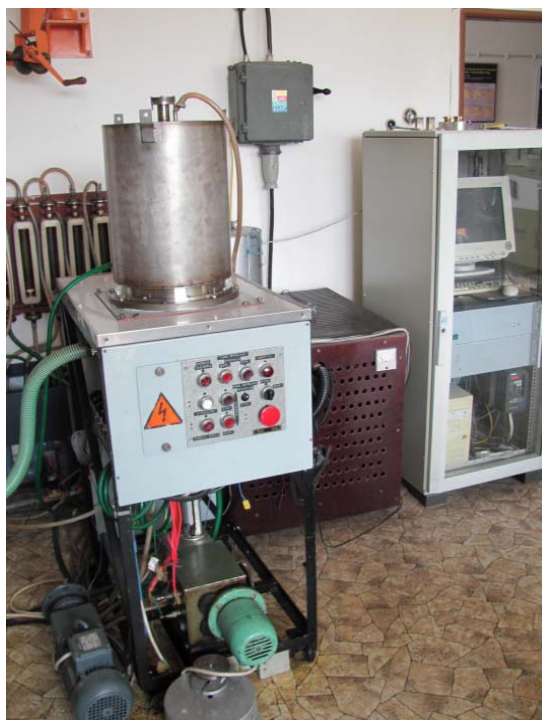
Fig. 2. Computer controlled Bridgman type apparatus designed for ground based solidification and CET experiments of TiAl based alloys.
