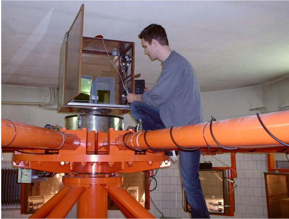
Fig. 10. Installation of the control part of a telemetric system on the centrifuge central axis
