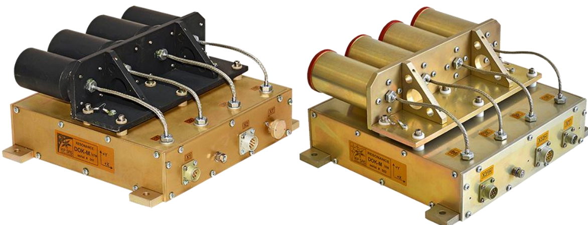
Figure 1.6. The structural thermal model DOK-M/STM and engineering model DOK-M/EM are undergoing testing at Space Research Institute, Moscow.
