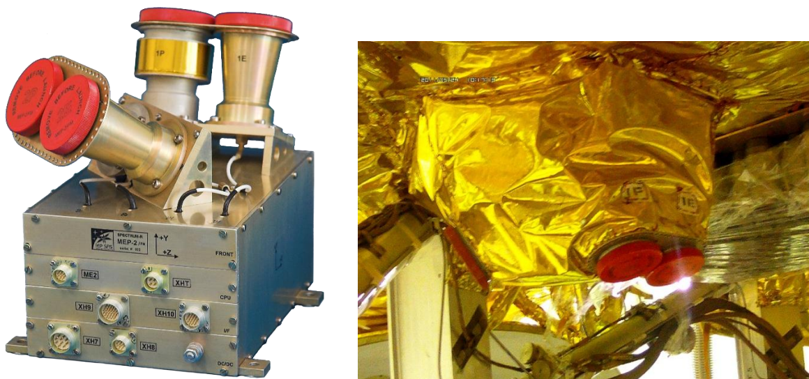
Figure 1.2. Energetic particle spectrometer MEP-2. The configuration on delivery and after installation on board of the space observatory Spektr-R (Radioastron).
