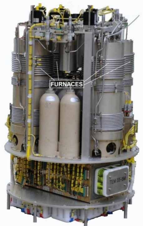
Figure 4.4. IMPRESS module consisting of four furnaces for directional solidification in microgravity conditions.
