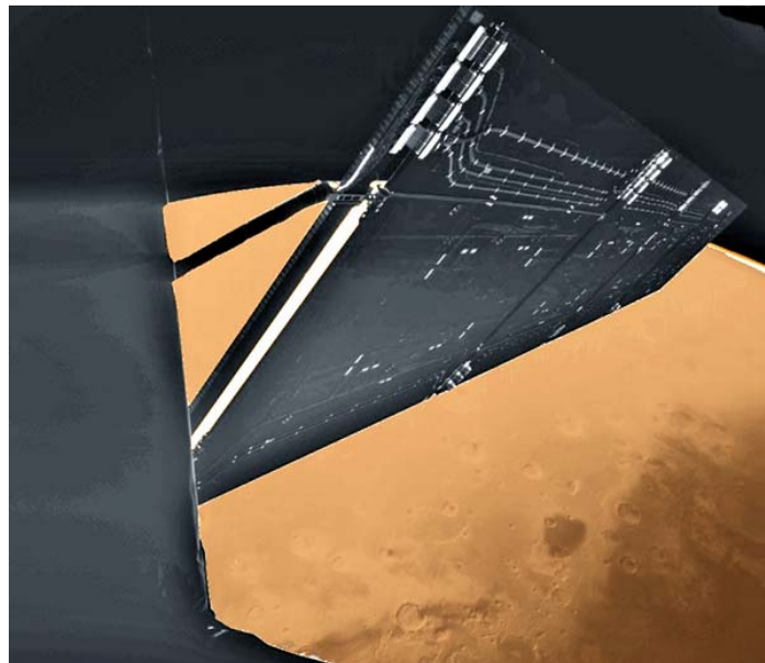
Fig.3. Flyby of the ROSETTA spacecraft around planet Mars in February 2007. The image of the Mars surface was provided by CIVA camera on board of Lander Philae and transferred to Orbiter via umbilical link under ESS data management (Credit: ESA)
