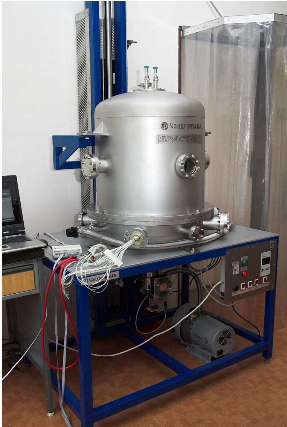
Fig.4. The space environment simulator SPACEVAC has been developed and manufactured in cooperation with Vacuum Praha company for environmental testing and qualification of spaceborn instrumentation that are under development at Institute of Experimental Physics. The SPACEVAC consists of a bell vacuum chamber equipped with dry pumping system (scroll pump + turbomolecular pump), temperature-controlled mounting platform and temperature-controlled background radiation shroud. Support by APVV grant agency, project 00538 is acknowledged.
